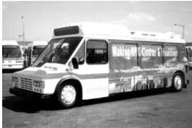
This hybrid bus runs on batteries that get their charge from an internal combustion engine fueled by compressed natural gas. It was developed with funding from the New York State Energy Research and Development Authority and tested in the mid-'90s at seven transit agencies throughout New York State. The first hybrid electric-CNG bus to see real-world transit service, it confirmed the viability of this clean-fuel technology.
